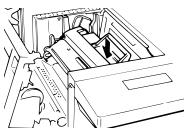
Swing the printer cover back down. Push down on a portion of the cover to lock the cover into its normal position.
